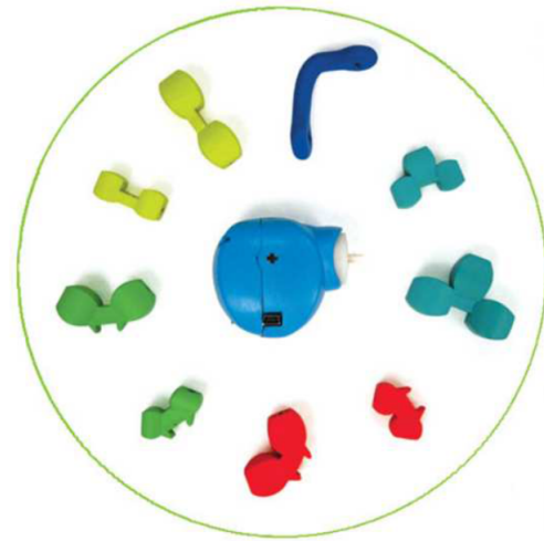
Figure 1: An example of an assembled and unassembled Topobo creature
