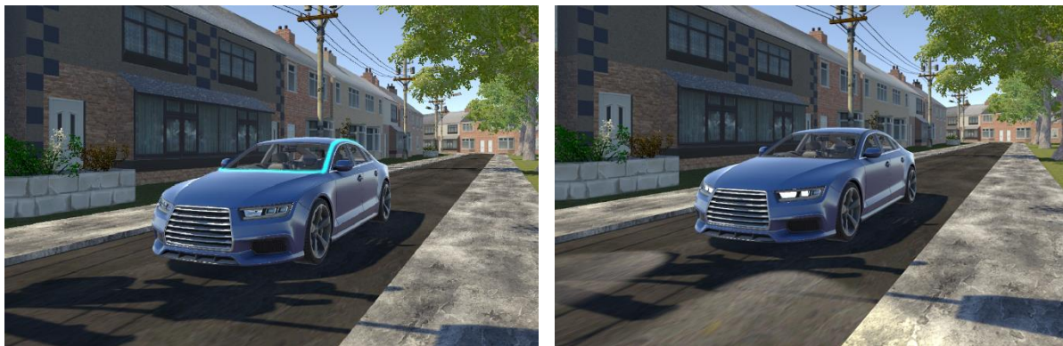
Figure 3. The two eHMI used for this study: Slow Pulsing Light Band (left) and the Flashing Headlight (right) eHMI
